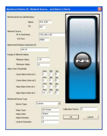
The AC Power probe reports 0 when voltage is normal and 1 when the power is off. A minimum value of -10 and a maximum value of 0 are the recommended allowed value ranges. You could use -20 or -50 as the minimum value but the maximum value must be 0. The probe's power-off value of "1" response will be out-of-range which will eventually elicit an alarm.
