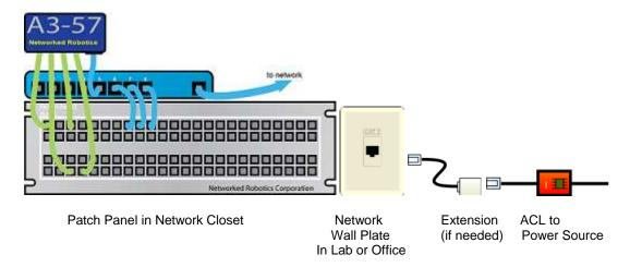
In the case above the connection to the wall power socket is "patched in" via your building's CATx cable plant and network wall jacks (see figure below). In this case the power supplying NTMS hardware is remote from the outlet in the lab or office.
