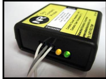
Secure the DCP to a convenient location using the dual-lock provided on the back of the DCP. The dual-lock adheres to metal or plastic surfaces. It is not designed to adhere to porous surfaces such as drywall or wood.
