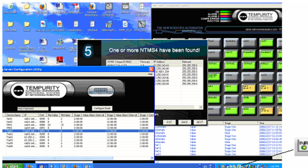
Figure 1: The 3 Main Software Components of the Tempurity System Running Simultaneously on a Single Computer
