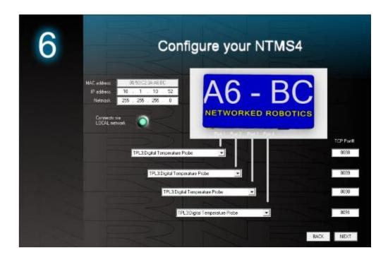
4. Click on the drop-down for the physical port on the NTMS where the probe is connected, and under the "Device Type" drop down, select TPL3.
