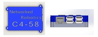
The adapter is connected to any of the four USB ports on the NTMS4p. The TPL3-series phone-style connector is plugged into the adapter. The NTMS4p supports wired or wireless data acquisition.
