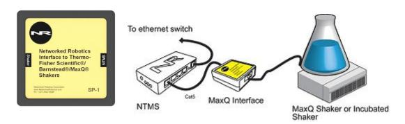
The MaxQ line has both digital and analog versions of each model. This product is compatible with the digital-version models, all of which have serial data ports for data output. Digital versions comprise the E-series and have "SHKE" model numbers. The SHKE 420, 481, 2000, 4000, 4450, 5000, and 7000 models support the use of this product. This interface is not appropriate for use with the A-series (analog) versions of the MaxQ line.
