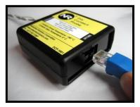
Replace the cover and its screws to close the DCP. Then use the provided CAT5E cable to connect the DCP to any of the four probe ports on the NTMS. If needed, you can use a longer length of CAT5 cable. The maximum distance, however, should not exceed 100 meters.
