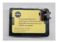
Connect the standard Cat5 cable from the top-mounted RJ45-jack on the interface labeled "NTMS" to one of the NTMS data jacks.
