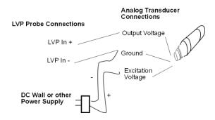
Transducer output is connected to the Low Voltage Probe as shown below:
