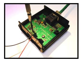
Attach the negative or ground wire of the sensor's output voltage to the screw terminal labeled (IN-) on the Voltage Probe board. This is the leftmost pin when facing the LEDS.
